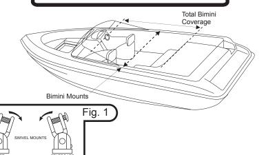
Determine what area of the boat you want to cover with the bimini. Bimini swivel mount locations are approximately half the distance of the total length of the bimini. Measure for mount placement and mark. Make sure the swivel mounts are parallel to each other and facing with the swivel movement going toward inside of boat (See Fig.1).
