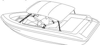
With bimini secure in the mounts, open the bimini and determine the best position for the hold down strap eyes. Strap eyes should be mounted to a flat surface whenever possible and straps should maintain an angle between 30 and 60 degrees from front to rear. To minimize side to side movement, it is suggested to mount front strap eyes as far inboard as allowable. Line up strap eyes across the boat.
