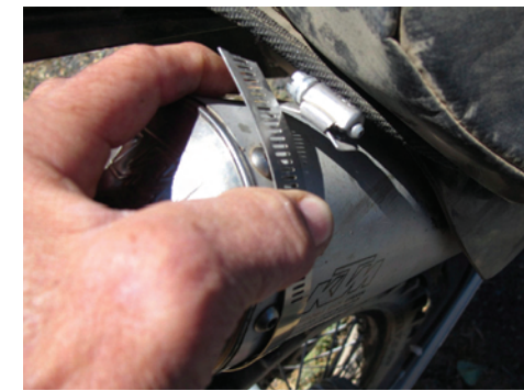
Trim excess hose clamp on smaller diameter exhaust pipes.
