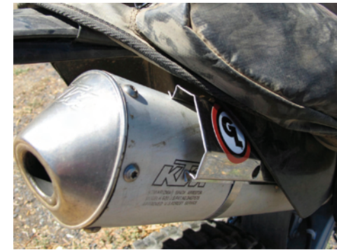
Position Hot Spring Heat Shield between side panel plastic and exhaust. On some newer model motorcycles, the shield may be positioned beyond the side panel to keep the saddlebag from touching the exhaust.
