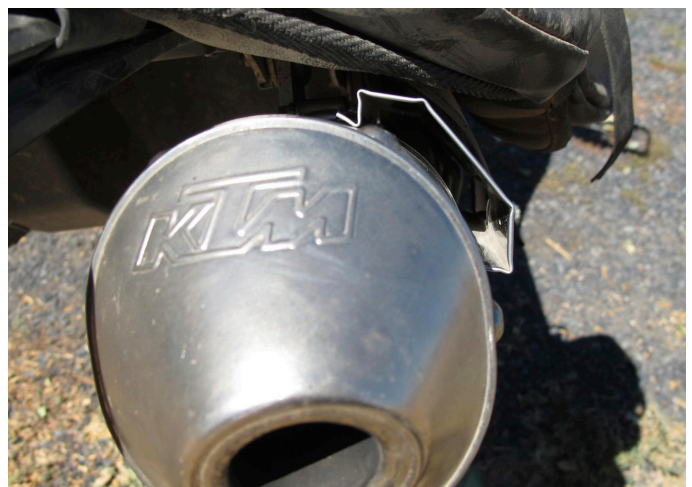
Air will pass through the correctly installed shield and no melting will occur.
