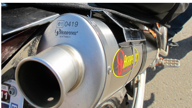
Dual exhaust motorcycles require a shield on each muffler.
