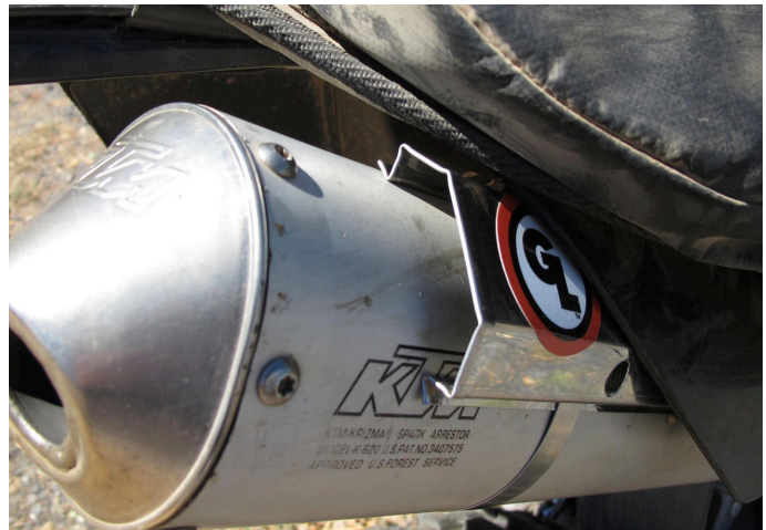
Position Hot Spring Heat Shield between side panel plastic and exhaust. On some newer model motorcycles, the shield may be positioned beyond the side panel to keep the saddlebag from touching the exhaust.
