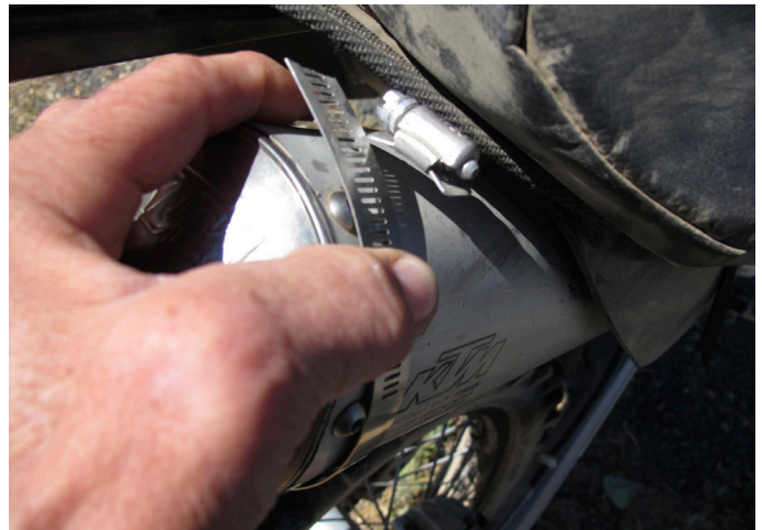
Trim excess hose clamp on smaller diameter exhaust pipes.
