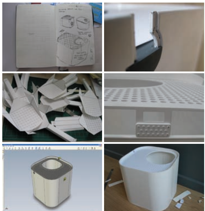
(Above) The ModBox is a stylish alternative to the traditional cat litter tray (Below) Clockwise from top left: Initial Sketches, Prototype hinge, Prototype lock, Foam core mock-up, SolidWorks model, Scoop studies
