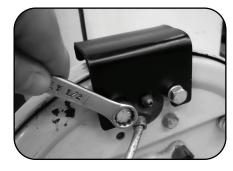
Remove the two bolts that hold the wheel cylinder to the backing plate, and install the retainer using the bolts, spacers and lockwashers supplied in the kit.
