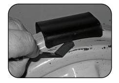
Check the clearance between the retainer and the drum, all around the circumference of the drum as you rotate it. Clearance should be 0.080 inch at all locations. If necessary file or grind the edge of the retainer to privide the required clearance.
