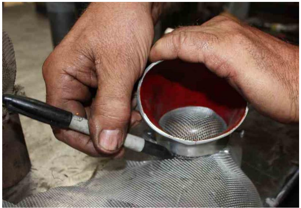
Step 4. Cut the screen to size.
