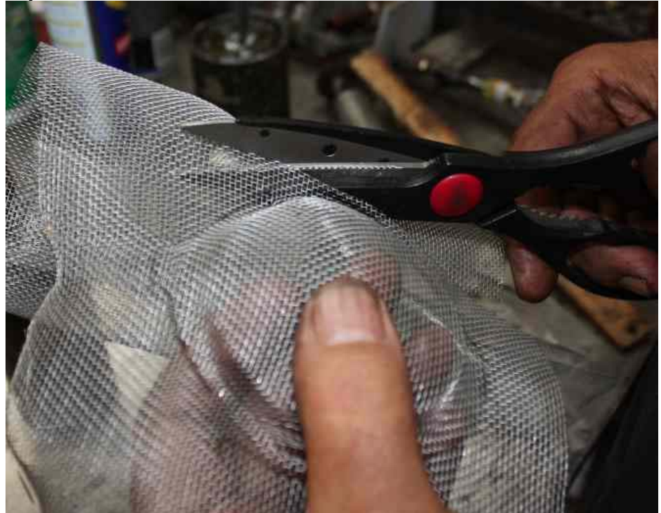
Step 5. Install the screen and riser. You may need to re-cut the screen if any excess is hanging outside of the riser.
